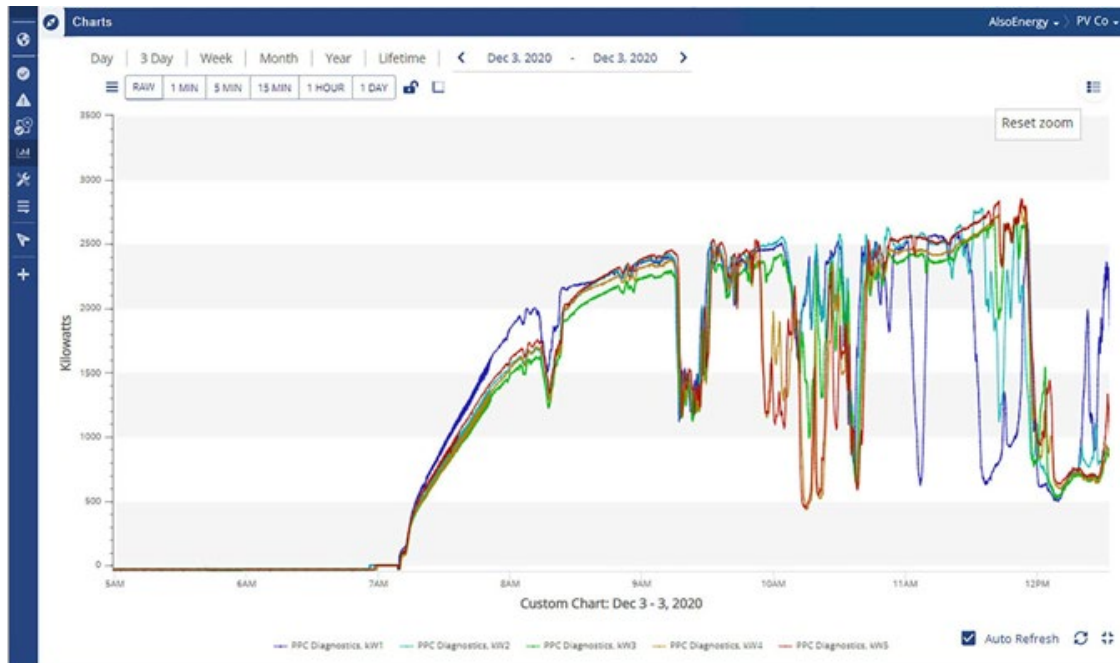
Fig. 1 Central inverters reacting to variable spatial irradiance. Actual site data, Hawaii
