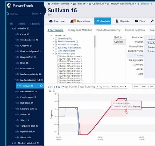
Interactive, built-in charting, such as tracker angle and RMS error, actual versus modeled production, and more, help analyze performance deviations while customized charting enables selection of specific hardware registers and aggregation methods.
