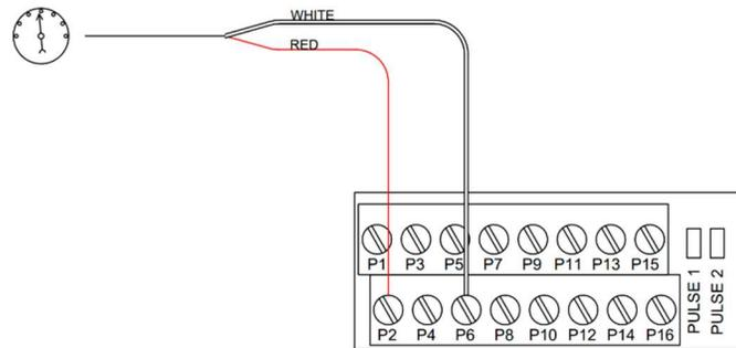
Figure 34: Pressure Sensor Wiring to IWS
