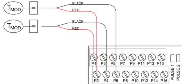
Figure 29: Loop-Powered Module Temperature Sensor Wiring to IWS
