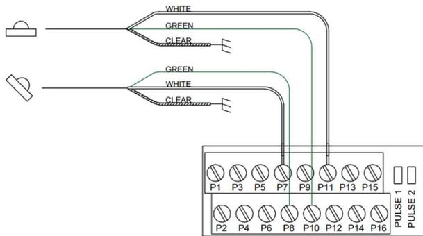
Figure 33: Apogee Analog Pyranometer Wiring to IWS
