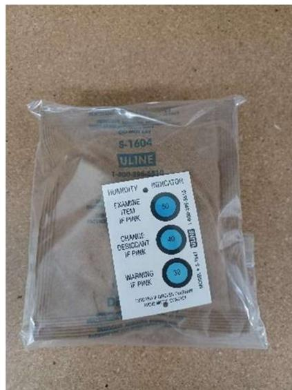
Figure 5: Desiccant Pack in Plastic Wrapper
