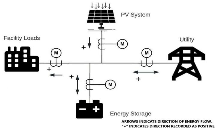
Figure 12: Metering Diagram
