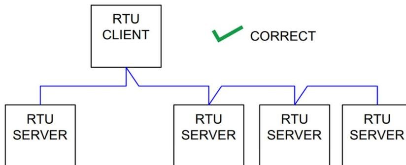
Figure 10: Example of Correct Daisy Chain Configuration
