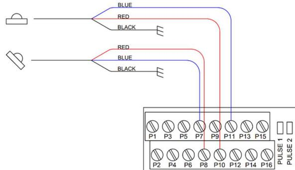
Figure 32: Kipp & Zonen Analog Pyranometer Wiring to IWS
