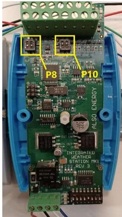
Figure 43: IWS Board Highlighting Gain Switches
