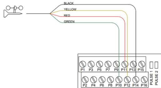
Figure 26: Davis Anemometer Wiring to IWS
