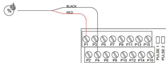
Figure 31: BAPI Humidity Sensor Wiring to IWS
