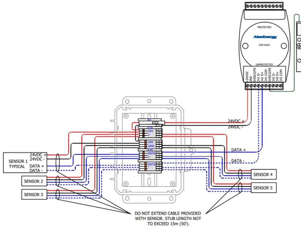
Figure 38: AlsoEnergy Weather Station Junction Box Connections
