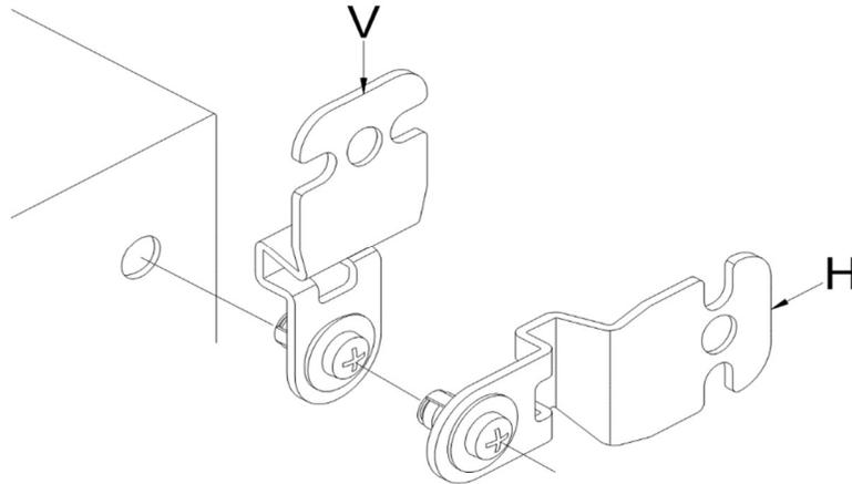
Figure 4: Mounting Brackets Shown in Vertical and Horizontal Positions
