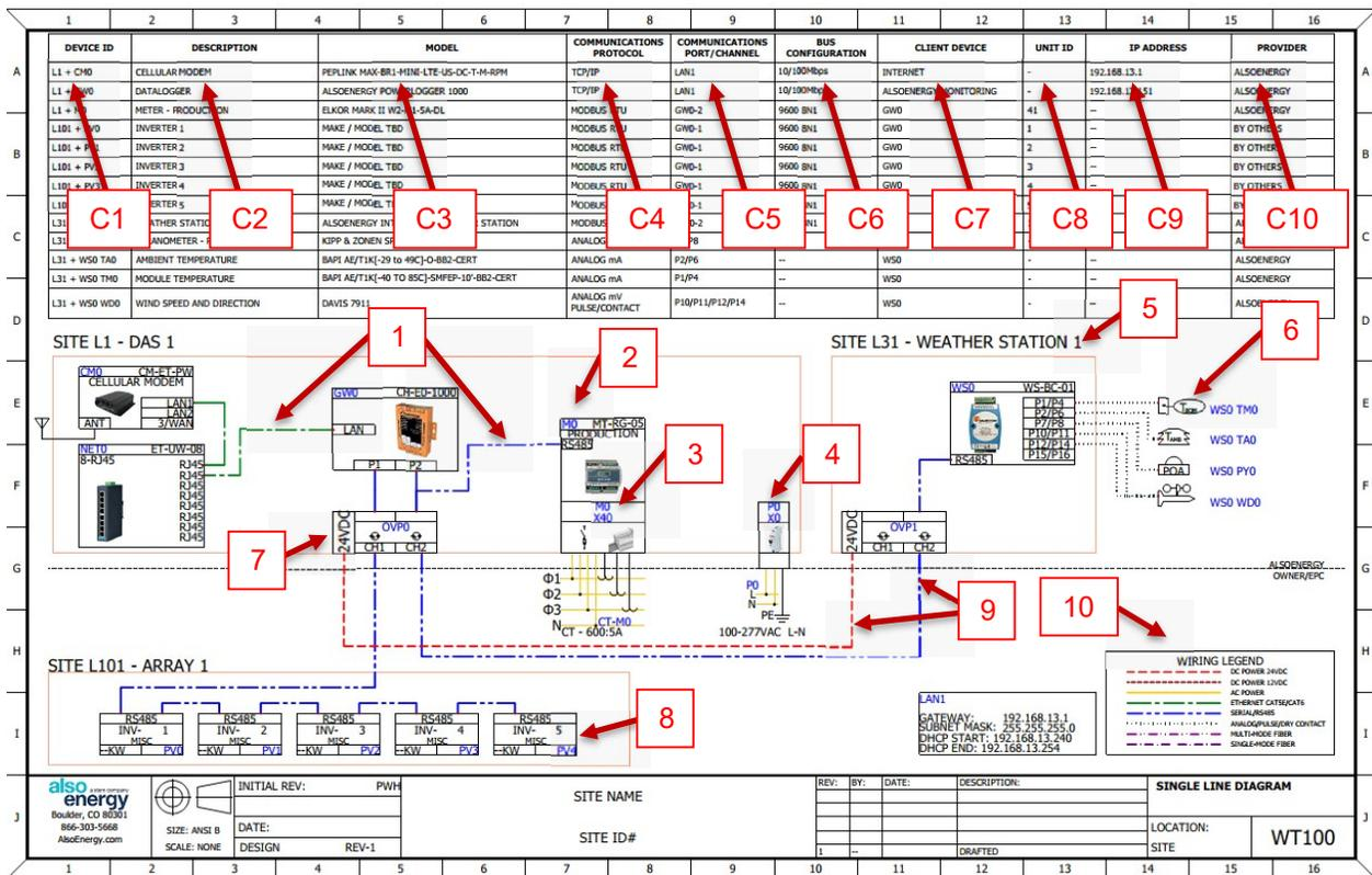
Figure 2: Single Line Diagram and Communications Table
