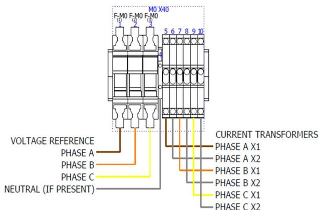
Figure 16: Field Wiring of Meter Interface Block
