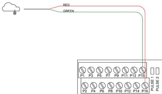
Figure 27: Davis Rain Collector Wiring to IWS
