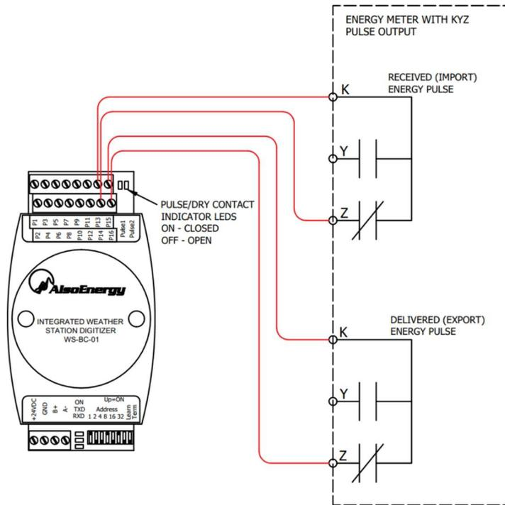
Connect K and Z terminals as shown in [Figure 41](#) and [Table 19](#). The Y contact is not used.
