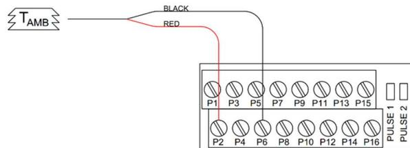
Figure 30: Loop-Powered Ambient Temperature Sensor Wiring to IWS
