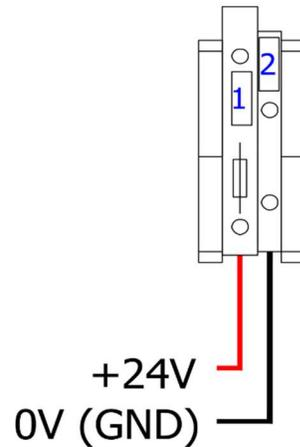
Figure 8: 24 VDC Fused Output without OVP
