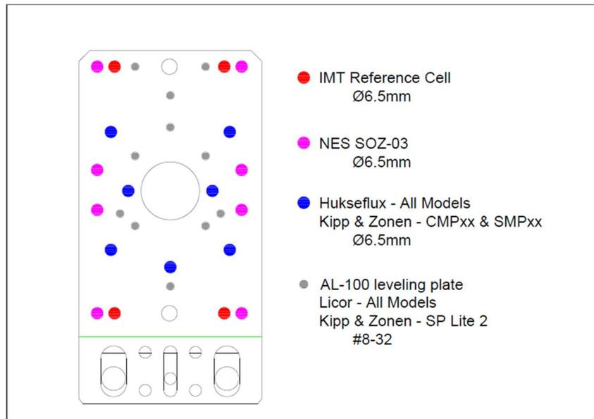
Figure 22: Mounting Holes for Select Pyranometers and Sensors
