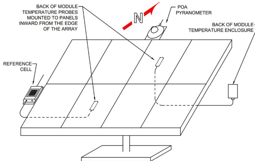
Figure 19: Examples of Sensors Mounting on a PV Array
