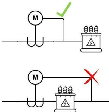
The location of CTs can vary depending on the site. Refer to the site documentation to determine the CT location. They should be placed in the same general location as voltage taps (they must be on the same side of the transformer) and in a location that captures all intended production (around all feeders associated with the metered circuit). Service panels and AC disconnect cabinets typically supply ample space and weather protection for CTs.
